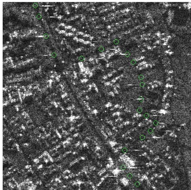
Figure 2: Simulated SAR image of urban area with moving targets. Original target positions denoted by green circles.
